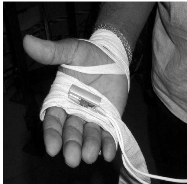
Figure 2 Accelerometer package inserted into his handwrap and used to measure the boxer's hand motion. Photograph reproduced with patient consent.
