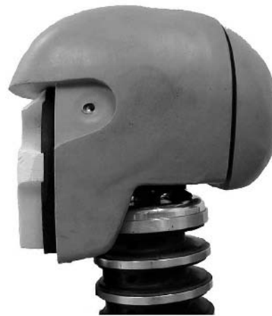
Figure 1 Test fixture with Hybrid III dummy attached. Image on the right is a breakout of the Hybrid III headform with frangible face foam subassembly exposed.
