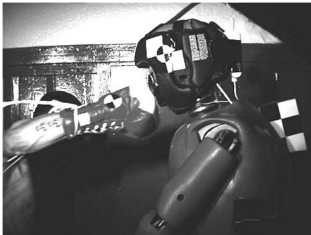
Figure 3 Olympic boxer throwing straight right punch to jaw region of instrumented Hybrid III dummy.
